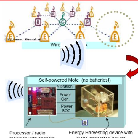
Processor / radio modules with sensors and signal conditioning Energy Harvesting device with piezo generator, power conversion electronics, & power storage module
